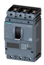
circuit breaker 3VA2 IEC frame 250 breaking capacity class C Icu=110kA @ 415V 3-pole, motor protection ETU860M, LSIG, In=200A overload protection Ir=80A...200A short-circuit protection Isd=1.2..15x In, Ii=3..15x In gr.-fault prot., can be sw. off Ig=0.2...1 x In, tg=0.05-0.8s nut keeper kit
