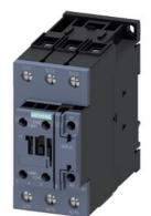
power contactor, AC-3e/AC-3, 51 A, 22 kW / 400 V, 3-pole, 20-33 V AC/DC, 50/60 Hz, with integrated varistor, auxiliary contacts: 1 NO + 1 NC, screw terminal
