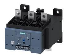
Overload relay 50...200 A for motor protection Size S6, Class 10E Contactor mounting/stand-alone installation Main circuit: busbar connection Auxiliary circuit: Screw terminal Manual-Automatic-Reset
