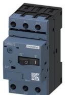
Circuit breaker size S00 for motor protection, CLASS 10 A-release 0.28...0.4 A N-release 5.2 A Screw terminal Standard switching capacity
