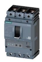
circuit breaker 3VA2 IEC frame 160 breaking capacity class C Icu=110kA @ 415V 3-pole, line protection ETU330, LIG, In=160A overload protection Ir=63A...160A short-circuit protection Ii=1.5...10 x In ground-fault protection Ig=0.2...1 x In, tg=0.1/0.3s nut keeper kit
