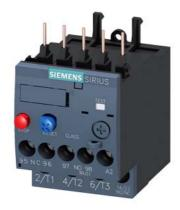
Overload relay 4.5...6.3 A Thermal For motor protection Size S00, Class 10 Contactor mounting Main circuit: Screw Auxiliary circuit: Screw Manual-Automatic-Reset
