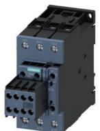
power contactor, AC-3e/AC-3, 65 A, 30 kW / 400 V, 3-pole, 83-155 V AC/DC, 50/60 Hz, with integrated varistor, auxiliary contacts: 2 NO + 2 NC, screw terminal, removable auxiliary switch
