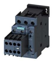
power contactor, AC-3e/AC-3, 25 A, 11 kW / 400 V, 3-pole, 110 V AC, 50 Hz, auxiliary contacts: 2 NO + 2 NC, screw terminal, removable auxiliary switch
