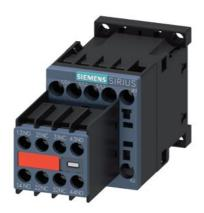
power contactor, AC-3e/AC-3, 12 A, 5.5 kW / 400 V, 3-pole, 230 V AC, 50/60 Hz, auxiliary contacts: 2 NO + 2 NC, screw terminal, captive auxiliary switch
