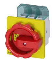
SENTRON, Switch disconnector 3LD, emergency switching-off switch, 3-pole, Iu: 32 A, operating power / at AC-23 A 400 V: 11.5 kW, front-mounted, rotary operating mechanism, Red / yellow, 4-hole mounting of the handle
