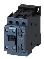
power contactor, AC-3e/AC-3, 32 A, 15 kW / 400 V, 3-pole, 24 V DC, 0.7-1.25\* Us, with plugged-in varistor, auxiliary contacts: 1 NO + 1 NC, screw terminal, suitable for PLC outputs, not expandable with auxiliary switch
