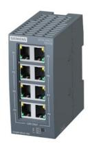
SCALANCE XB008 Unmanaged Industrial Ethernet Switch for 10/100 Mbit/s; for setting up small star and line topologies; LED diagnostics, IP20, 24 V AC/DC power supply, with 8x 10/100 Mbit/s twisted pair ports with RJ45 sockets; Manual available as a download.
