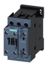
power contactor, AC-3e/AC-3, 25 A, 11 kW / 400 V, 3-pole, 110 V AC, 50/60 Hz, auxiliary contacts: 1 NO + 1 NC, screw terminal
