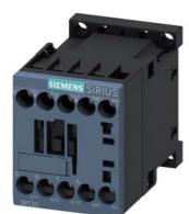
power contactor, AC-3e/AC-3, 7 A, 3 kW / 400 V, 3-pole, 12 V DC, auxiliary contacts: 1 NC, screw terminal
