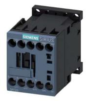
power contactor, AC-3e/AC-3, 9 A, 4 kW / 400 V, 3-pole, 24 V DC, auxiliary contacts: 1 NC, screw terminal
