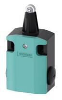
Position switch Metal enclosure 56 mm wide, Device connection 3x (M20x 1.5) 1 NO/1 NC quick action contacts, Roller plunger with 3 mm overtravel, Stainless steel roller 13 mm
