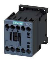
power contactor, AC-3e/AC-3, 7 A, 3 kW / 400 V, 3-pole, 24 V DC, auxiliary contacts: 1 NC, screw terminal, communication-capable
