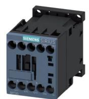
power contactor, AC-3e/AC-3, 16 A, 7.5 kW / 400 V, 3-pole, 230 V AC, 50/60 Hz, auxiliary contacts: 1 NC, screw terminal
