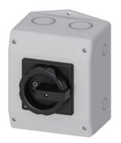
SENTRON, Switch disconnector 3LD, main switch, 3-pole, lu: 63 A, Operating power / at AC-23 A at 400 V: 22 kW, molded-plastic encapsulation for metric cable gland, rotary operating mechanism, black
