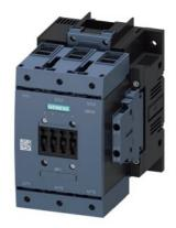
power contactor, AC-3e/AC-3 115 A, 55 kW / 400 V, AC (50-60 Hz) / DC Uc: 23-26 V 3-pole, auxiliary contacts 2 NO + 2 NC drive: conventional main circuit: box terminal control and auxiliary circuit: screw terminal
