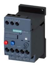
Overload relay 1.8...2.5 A Thermal For motor protection Size S00, Class 10 Stand-alone installation Main circuit: Screw Auxiliary circuit: Screw Manual-Automatic-Reset
