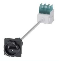
SENTRON, Switch disconnector 3LD, main switch, 3-pole, lu: 32 A, Operating power / at AC-23 A at 400 V: 11.5 kW, floor mounting with door coupling, rotary operating mechanism, black, 4-hole mounting of the handle
