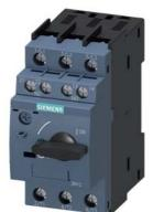
Circuit breaker size S0 for motor protection, CLASS 10 A-release 1.8...2.5 A N-release 33 A screw terminal Standard switching capacity with transverse auxiliary switches 1 NO+1 NC  $\,$
