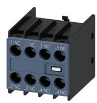
Auxiliary switch on the front, 2 NO + 2 NC Current path 1 NC, 1 NC, 1 NO, 1 NO for 3RH and 3RT screw terminal .1/.2, .1/.2, .3/.4, .3/.4
