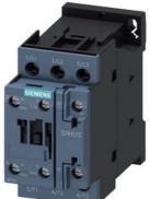
power contactor, AC-3e/AC-3, 9 A, 4 kW / 400 V, 3-pole, 110 V AC, 50 Hz / 120 V, 60 Hz, auxiliary contacts: 1 NO + 1 NC, screw terminal
