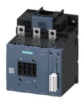
power contactor, AC-3e/AC-3 150 A, 75 kW / 400 V AC (50-60 Hz) / DC Uc: 200-277 V PLC input 24 V DC 3-pole, auxiliary contacts 1 NO + 1 NC drive: electronic main circuit: busbar control and auxiliary circuit: screw terminal with remaining lifetime indicator
