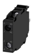
Contact module with 2 contact elements, 1 NO+1 NC, screw terminal, for front plate mounting
