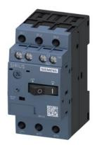
Circuit breaker size S00 for motor protection, CLASS 10 A-release 5.5...8 A N-release 104 A 1 NO+1 NC transverse Screw terminal Standard switching capacity
