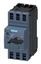
Circuit breaker size S00 for motor protection, CLASS 10 A-release 2.2...3.2 A N release 42 A Spring-type terminal Standard switching capacity
