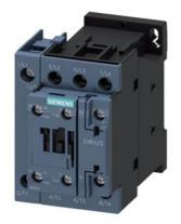
contactor AC-1, 50 A, 400 V / 40  $^{\circ}\text{C},$  4-pole, 230 V AC, 50/60 Hz, auxiliary contacts: 1 NO + 1 NC, screw terminal
