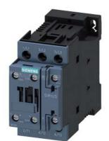
power contactor, AC-3e/AC-3, 12 A, 5.5 kW / 400 V, 3-pole, 24 V DC, 0.7-1.25\* Us, with plugged-in varistor, auxiliary contacts: 1 NO + 1 NC, screw terminal, suitable for PLC outputs, not expandable with auxiliary switch
