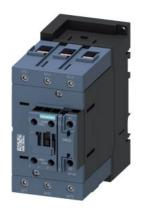
power contactor, AC-3e/AC-3, 95 A, 45 kW / 400 V, 3-pole, 110 V AC, 50/60 Hz, auxiliary contacts: 1 NO + 1 NC, screw terminal
