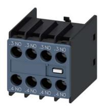
Auxiliary switch on the front, 4 NO Current path 1 NO, 1 NO, 1 NO, 1 NO for 3RH and 3RT screw terminal .3/.4, .3/.4, .3/.4, .3/.4
