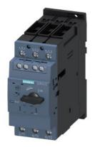
Circuit breaker size S2 for motor protection, CLASS 10 A-release 22...32 A N-release 416 A screw terminal Standard switching capacity with transverse auxiliary switches 1 NO+1 NC
