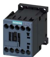
power contactor, AC-3e/AC-3, 9 A, 4 kW / 400 V, 3-pole, 24 V DC, auxiliary contacts: 1 NO, screw terminal, upright mounting position
