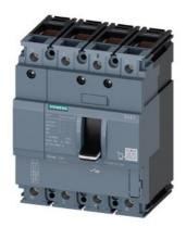
circuit breaker 3VA1 IEC frame 100 breaking capacity class B Icu=16kA @ 415V 4-pole, line protection TM210, FTFM, In=16A overload protection Ir=16A fixed short-circuit protection Ii=20 x In N conductor unprotected clamp connection
