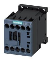
power contactor, AC-3e/AC-3, 9 A, 4 kW / 400 V, 3-pole, 110 V AC, 50/60 Hz, auxiliary contacts: 1 NC, screw terminal
