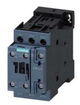
power contactor, AC-3e/AC-3, 38 A, 18.5 kW / 400 V, 3-pole, 24 V DC, auxiliary contacts: 1 NO + 1 NC, screw terminal
