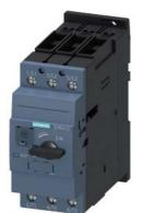
Circuit breaker size S2 for transformer protection A-release 18...25 A N-release 500 A screw terminal Standard switching capacity
