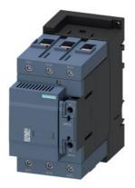
capacitor contactor, AC-6b 100 kVAr, / 400 V, 3-pole, 230 V AC, 50 Hz, auxiliary contacts: 1 NO + 1 NC, screw terminal
