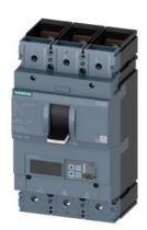
circuit breaker 3VA2 IEC frame 400 breaking capacity class C Icu=110kA @ 415V 3-pole, motor protection ETU860M, LSIG, In=250A overload protection Ir=100A...250A short-circuit protection Isd=1.2..15x In, Ii=3..15x In gr.-fault prot., can be sw. off Ig=0.2...1 x In, tg=0.05-0.8s nut keeper kit
