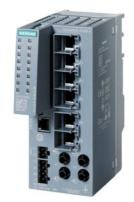
SCALANCE XC206-2 manageable Layer 2 IE switch; IEC 62443-4-2 certified; 6x 100 Mbit/s RJ45 ports; 2x 100 Mbit/s ST/BFOC ports; 1x console port; diagnostics LED; redundant power supply; temperature range -40 °C to +70 °C; assembly: DIN rail/S7 mounting rail/wall redundancy functions; office features (RSTP, VLAN,...); PROFINET IO device; Ethernet/IP-compliant C-PLUG slot;
