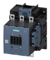
power contactor, AC-3e/AC-3 150 A, 75 kW / 400 V AC (50-60 Hz) / DC Uc: 220-240 V 3-pole, auxiliary contacts 2 NO + 2 NC drive: conventional main circuit: busbar control and auxiliary circuit: screw terminal
