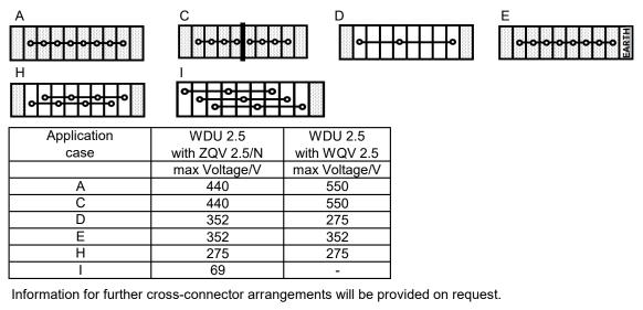
Max voltage data with optional screen bus bar LS 2,8:
