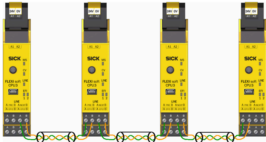
Figure 60: Connection of a Flexi-Line system
