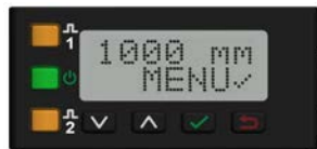
Figure 10. LE550 Display in Run Mode
