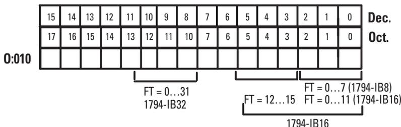
For example, to increase the off-to-on filter time to 4 ms for all inputs at address rack 1, module group 0 (using 1794-IB32, 1794-IB32K as an example), set the following bits and program.
