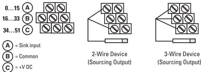
**Connect Wiring for the 1794-IB32 and 1794-IB32K using a 1794-TB32 or 1794-TB32S Terminal Base**
