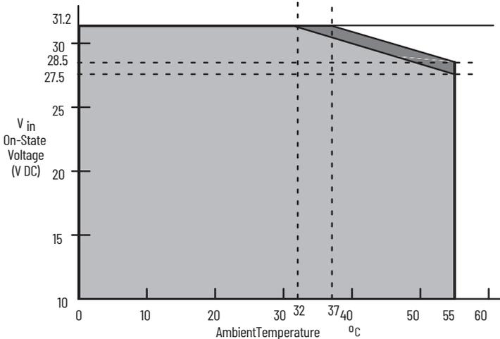
The area within the curve represents the safe operating range for the module under various conditions of user supplied 24V DC supply voltages and ambient temperature.
