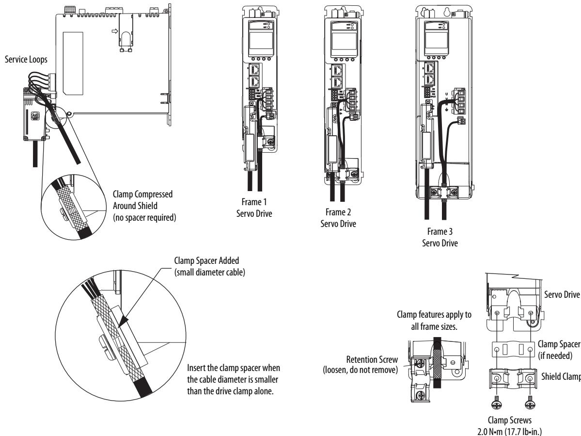
Refer to the Kinetix 5500 Servo Drives User Manual, publication [2198-UM001](#), for detailed information on wiring the 2198-H2DCK feedback converter kit and attaching the motor power/brake shield clamp.
