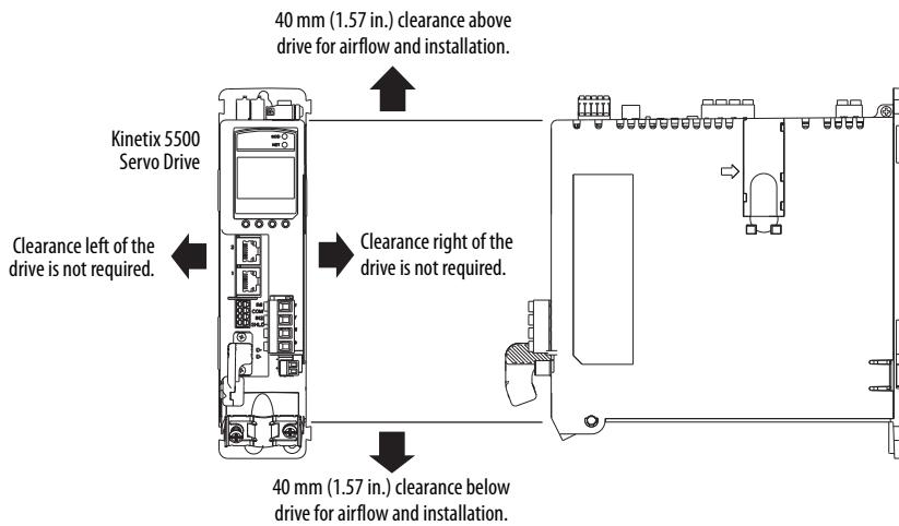
Refer to the Kinetix Servo Drives Technical Data, publication [GMC-TD003](#), for Kinetix 5500 drive dimensions.
