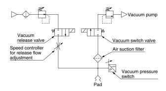
If a filter is required on the release pressure side, a different filter should be prepared.
