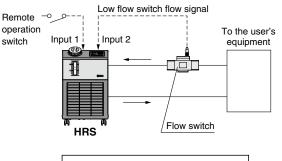
Power for flow switches (24 VDC) can be supplied by the thermo-chiller.
