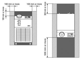
When option G, high-temperature environment specification, is selected: HRS030/HRS040/HRS050/HRS060 (A ventilation space is required since the ventilation slots are provided on the sides of the product.)
