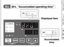
Displayed item Circulating fluid outlet temperature Circulating fluid return temperature Compressor gas temperature Circulating fluid outlet pressure Circulating fluid outlet pressure Compressor gas discharge pressure Compressor gas return pressure Accumulated operating time Accumulated operating time of pump Accumulated operating time of fan motor\*1 Accumulated operating time of compressor \*1 These are displayed only for air-cooled refrigeration.
