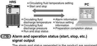
The alarm and status generated in the product are assigned to 3 output signals based on their contents, which can then be output.
