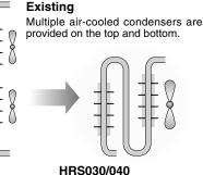
A maximum reduction in the height of the product has been achieved while expanding the cooling capacity by providing overlapped air-cooled condensers.
